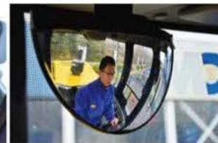
The super-large spherical rearview mirrors enlarge the visual field by 30%.
