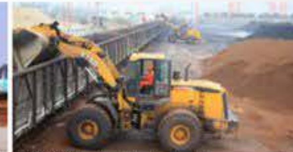
LW800K loader is loading lead zinc ore powder and coal powder in Wenzhou port
