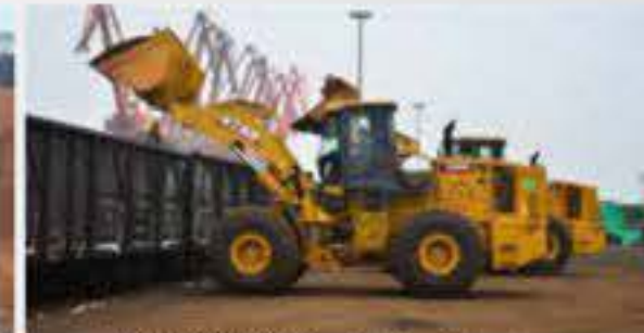
LW800K-LNG loader is loading iron powder in Tianjin port
