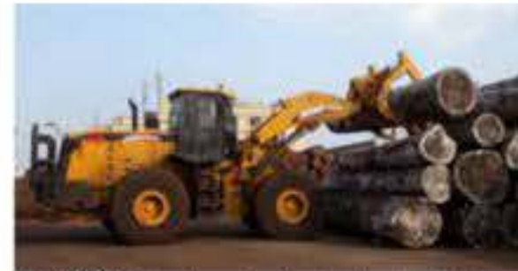
LW800K timber clamp loader is clamping timbers in Zhangjiagang port
