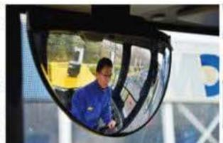
The super-large spherical rearview mirrors enlarge the visual field by 30%.
